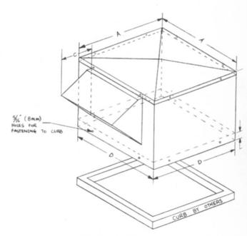
D is the inside dimension curb size must be smaller to allow for flashing.
